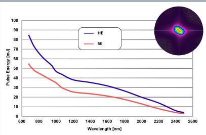
Typical far field beam profile at 750nm shown in insert.
